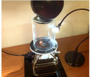
4. Place the chamber glass on top of the chamber platform.
